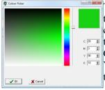
To choose a colour, move the slider up and down to the colour hue required. Then click on an exact colour in the main display. The colour patch at the top right will display the chosen colour and the CMYK colour value will be shown beneath that. You can also select the colour by directly entering the CMYK colour value.
